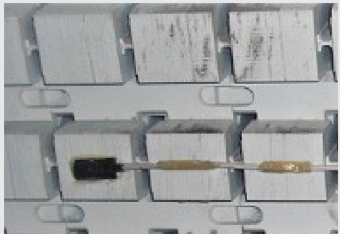
TF PROBE MOUNTED ON THE STATOR CORE
