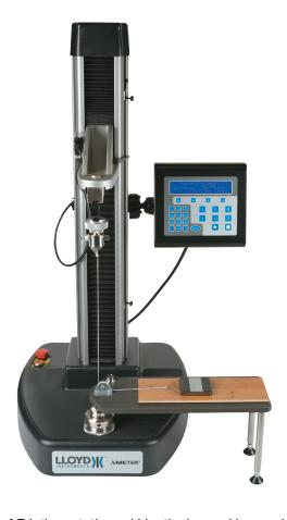
Coefficient of Friction, static and kinetic, is used in a variety of materials from lubricants, to films to household items (ceramic tiles) to determine the frictional characteristics of a material.
