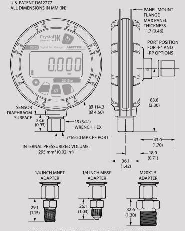
ADDITIONAL SENSOR LENGTH WITH OPTIONAL FITTING ADAPTERS
